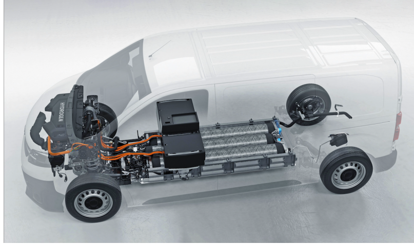
Figure 3.1: Opel Vivaro fuel cell powertrain [2]
