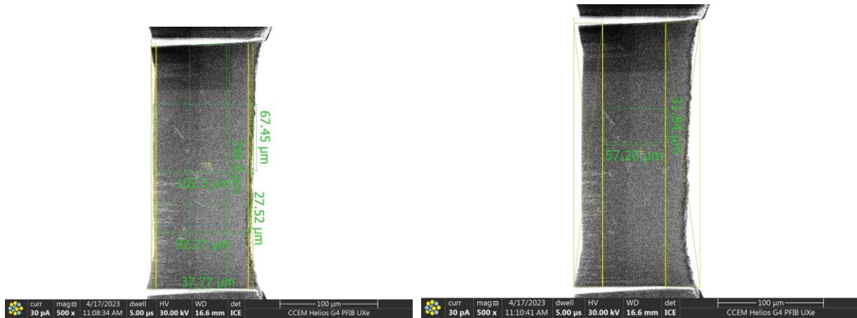
Figure 54: ISE images of gauge section of copper tensile specimen 3 from wedge 2 prior to cleaning of the edges. Left image shows centering of milling boxes using measurement boxes and right image shows final position of milling boxes prior to initiation of ion milling.
