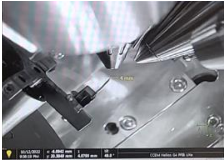
Figure 51: Specimen and stage configuration in Helios 5 Plasma-FIB chamber for thinning gauge sections of copper micro-tensile specimens.
