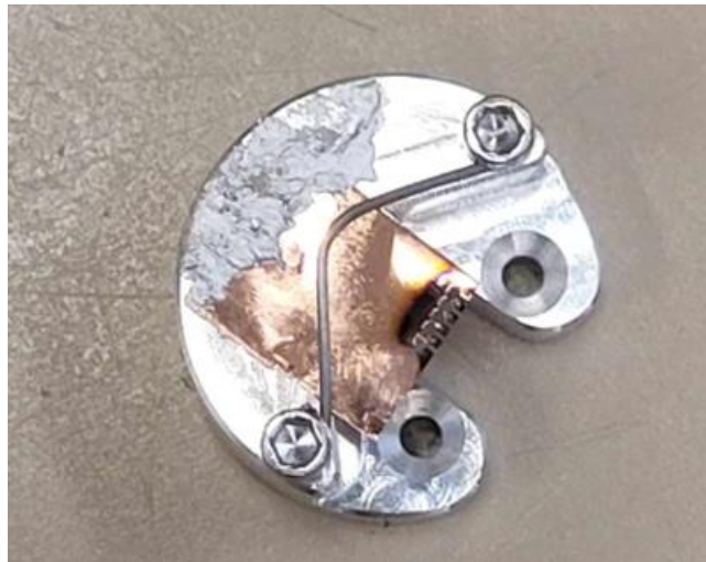
Figure 47: Copper wedge placed on the specimen holder prior to insertion into the custom-built micro-tensile bench.
