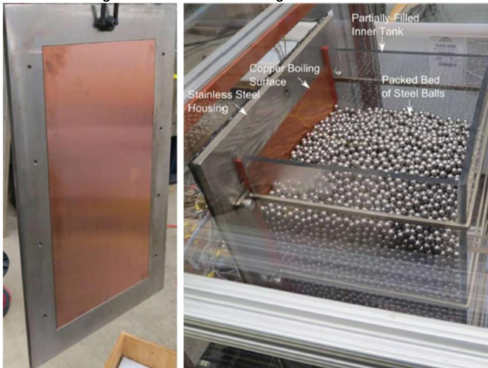
Figure 2: Heating Plate Assembled with Stainless Steel Housing (Left), and Installed in Apparatus during Test Preparations (Right) [5]
