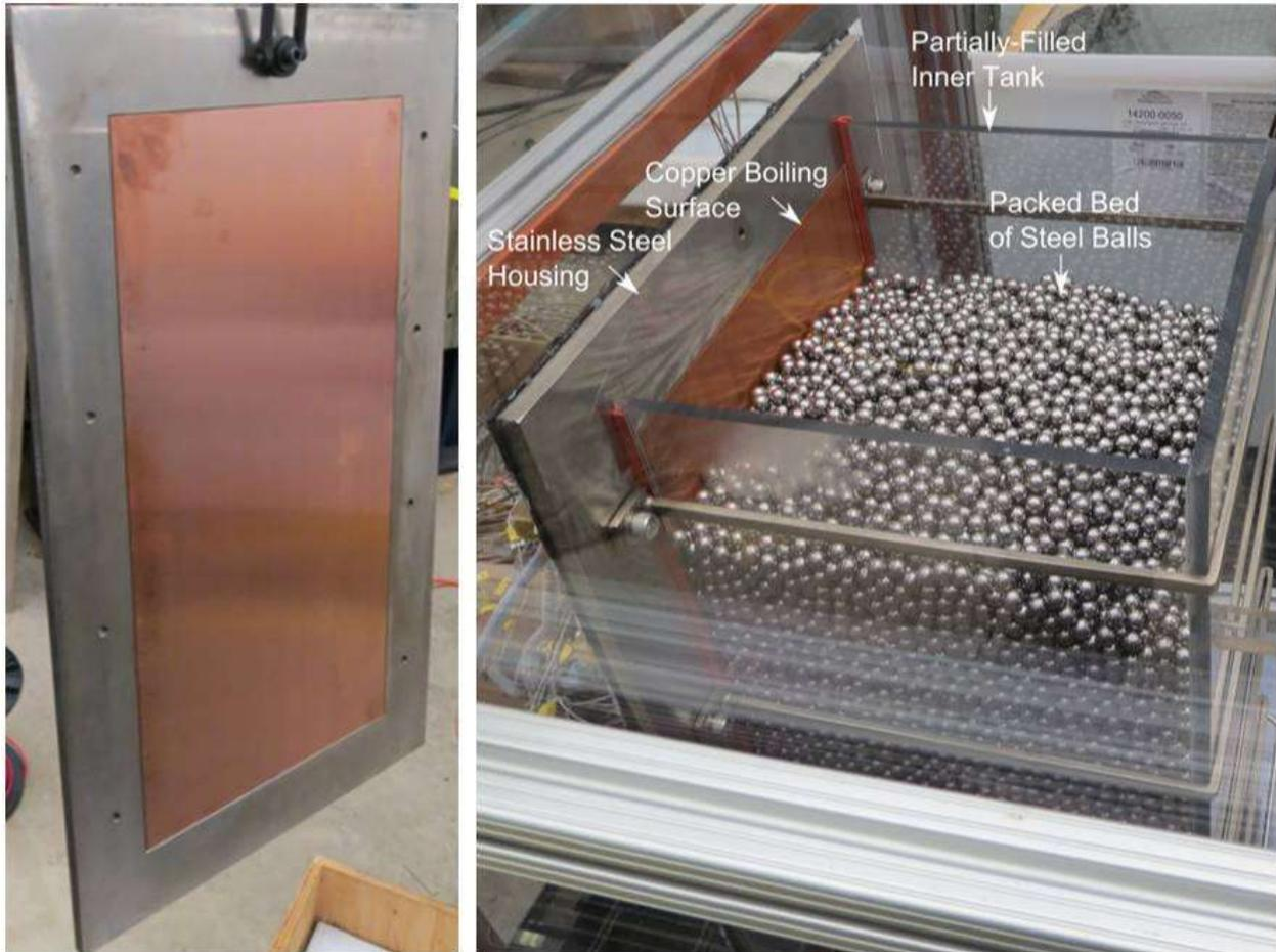
Figure 2. Heating Plate assembled with stainless steel housing (left), and installed in apparatus during test preparations (right).
