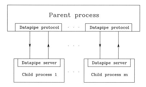
Datapipe interface between a parent process and a number of child processes
