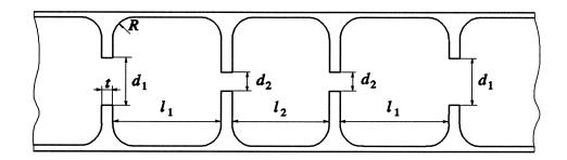
the waveguide cross-section:  $15.8 \times 7.9$  mm
