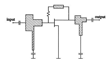
parameters of the feedback microstrip line and the microstrip T-structures
