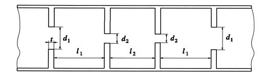
OS model (coarse model) for Space Mapping sharp corners
