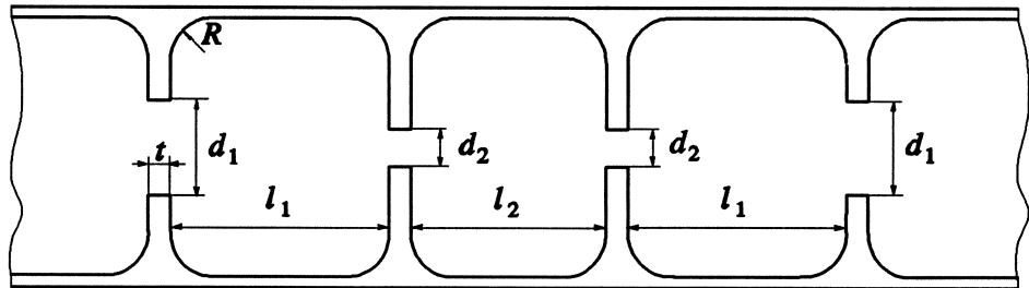
the waveguide cross-section is  $15.8 \times 7.9$  mm
