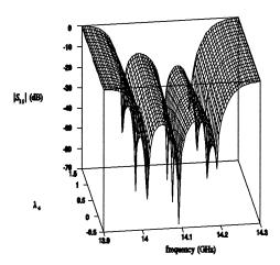
parameters varied in the range of the first aggressive SM step:  $\lambda_i = 0$  at  $x_{os}^*$  and  $\lambda_i = 1$  at  $x_{os}^1$
