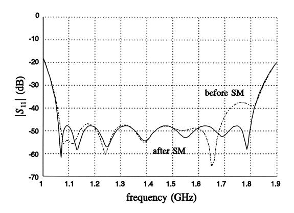
$|S_{11}|$  (dB) simulated by RWGMM before and after 14 steps of SM
