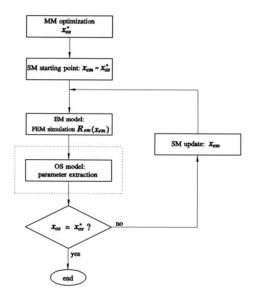
within the parameter extraction the Datapipe techniques can be utilized to connect external model simulators
