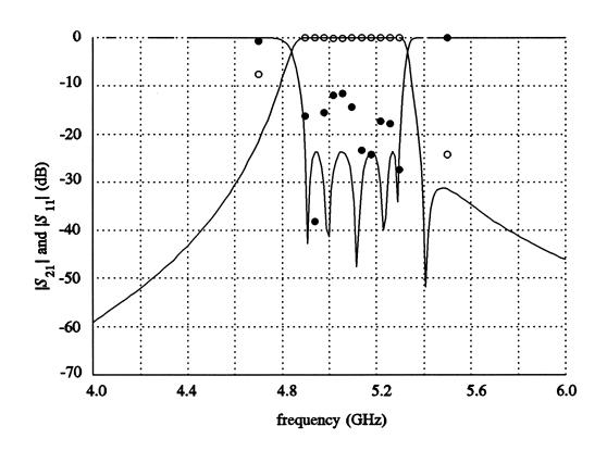
solid curves optimized  $|S_{11}|$  and  $|S_{21}|$  responses of the coarse model at the optimal point  $x_{os}^*$
