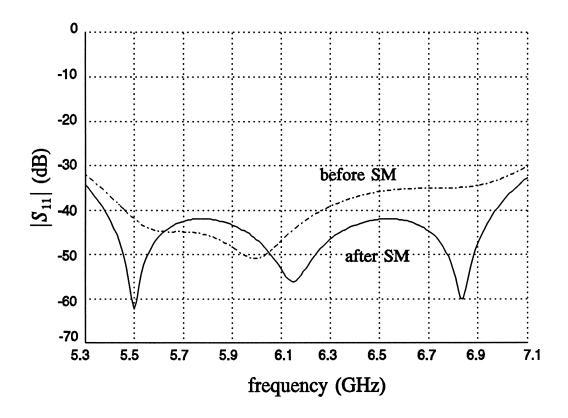
$|S_{11}|$  (dB) simulated by RWGMM before and after two steps of SM
