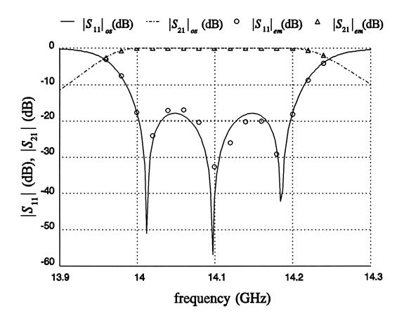
only 4 Maxwell Eminence simulations lead to the optimal solution
