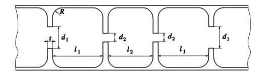
the waveguide cross-section is  $15.8 \times 7.9$  mm
