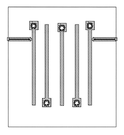
15 mil thick alumina substrate with  $\varepsilon_r = 9.8$ . the width of each microstrip is chosen to be 10 mil quarter wavelength resonators
