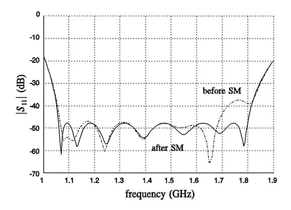
$|S_{11}|$  (dB) simulated by RWGMM before and after 14 steps of SM
