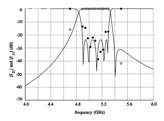
return loss is improved and the bandwidth is reduced at the lower frequency end
