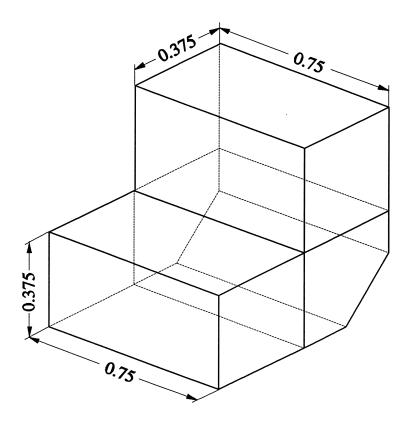
Fig. 1. Geometry of the optimized WR-75 mitered bend.
