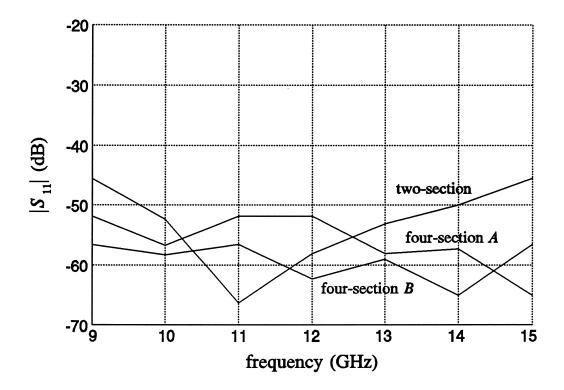
Fig. 9. Responses of optimized two- and four-section bends. The return losses are well above 40 dB (this is already in the simulator's noise level). The difference is due to the numerical approximation method and interpolation used.
