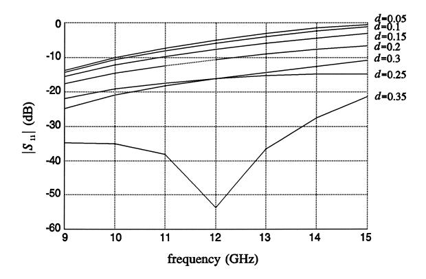
Fig. 3. Optimization using intuitive approach; d varied from 0.05 to 0.35 inches.
