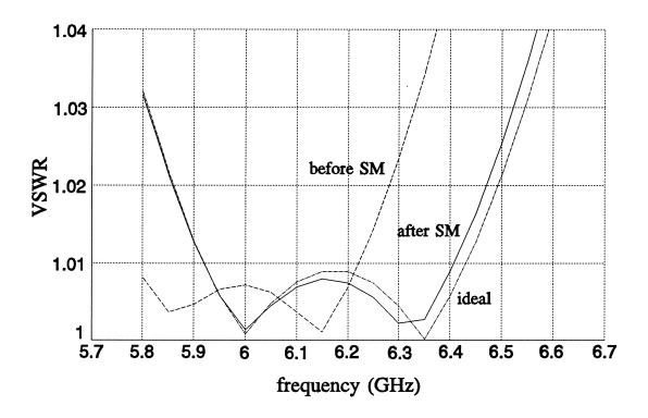
Fig. 14. VSWR response of a two-section waveguide transformer simulated by HFSS before and after 10 SM optimization iterations. Also shown is the optimal ideal response.
