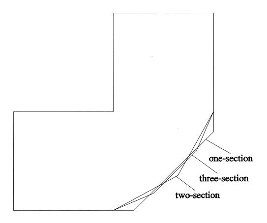
Fig. 6. Geometries of optimized one-, two- and three-section bends.
