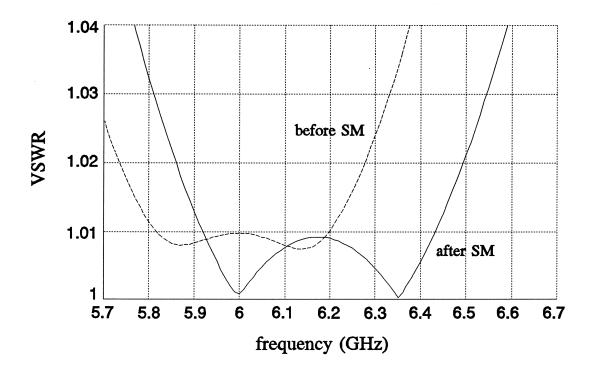
Fig. 11. VSWR response of a two-section waveguide transformer simulated using the nonideal model before and after SM optimization. The response after 7 SM iterations is indistinguishable from the optimal ideal response.
