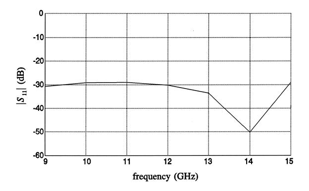
Fig. 4. Response of the optimized geometry of a single-section miter,  $d_{opt} = 0.2897$  inch.
