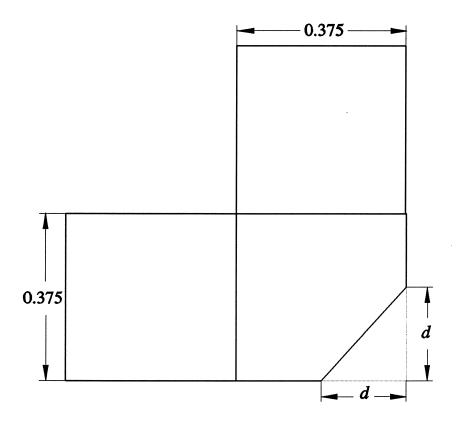
Fig. 2. Definition of the optimization variable d.
