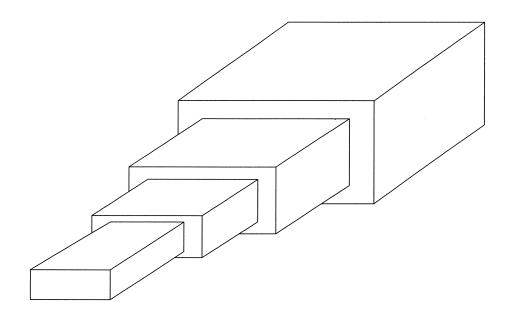
Fig. 10. A typical two-section waveguide transformer.
