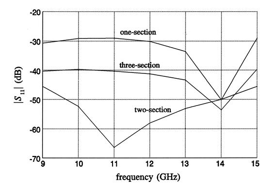
Fig. 7. Comparison of responses of optimized one-, two- and three-section mitered bends.
