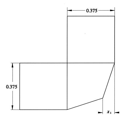
Fig. 5. Additional optimized geometries with optimization variables marked, (a) two-section miter, (b) three-section miter, (c) four-section miter, case A, (d) four-section miter, case B.
