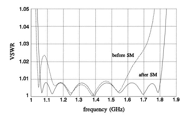
Fig. 13. VSWR response of a seven-section waveguide transformer simulated using the nonideal model before and after SM optimization. The response after 5 SM iterations is indistinguishable from the optimal ideal response.
