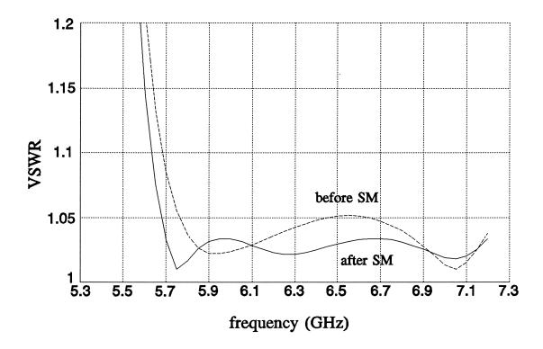
Fig. 12. VSWR response of a three-section waveguide transformer simulated using the nonideal model before and after SM optimization. The response after 6 SM iterations is indistinguishable from the optimal ideal response.
