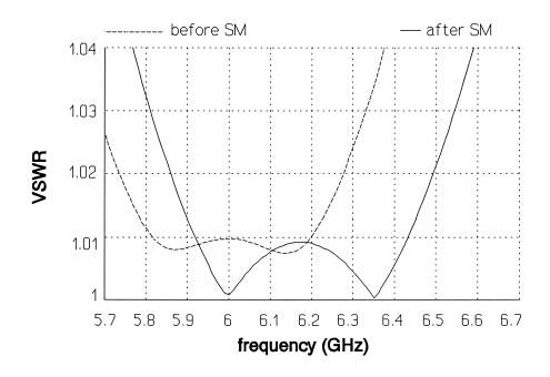
the response after 7 SM iterations is indistinguishable from the optimal ideal response
