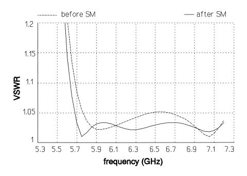
the response after 6 SM iterations is indistinguishable from the optimal ideal response
