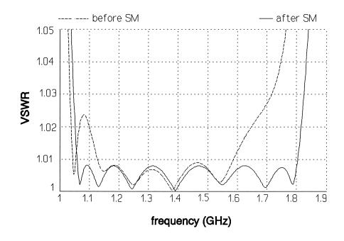
the response after 5 SM iterations is indistinguishable from the optimal ideal response
