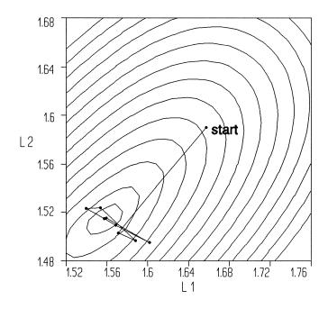
non-unique parameter extraction leads to the SM steps oscillating around the solution
