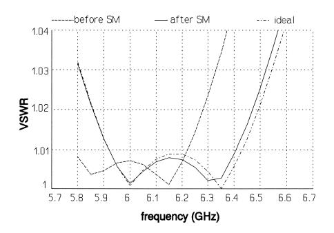
SM required 10 iterations (10 HFSS simulations) the solution is very close to the target ideal response
