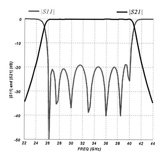
a typical minimax equal-ripple response of the filter was achieved after a series of consecutive optimizations with different subsets of optimization variables and frequency points
