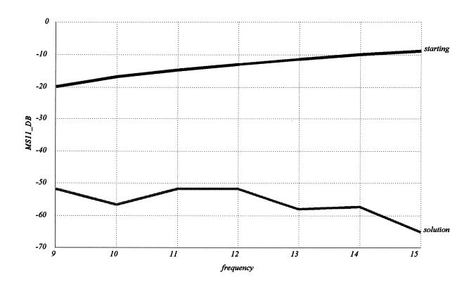
specification: return loss 40 dB from 9 to 15 GHz
