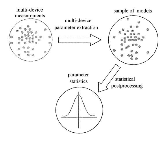
first, we extract model parameters for individual devices then the sample of model parameters is postprocessed to estimate the statistics
