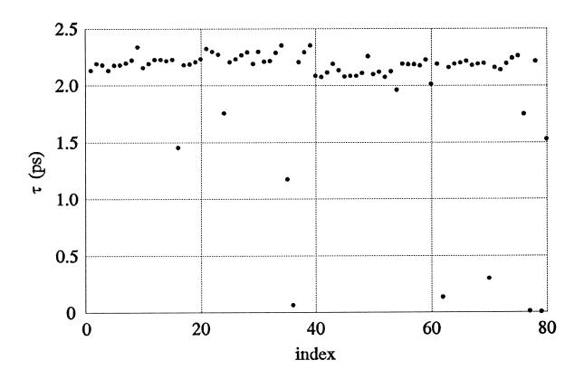
run chart of the extracted FET time-delay τ; a few abnormal values in the data due to faulty devices and/or gross measurement errors
