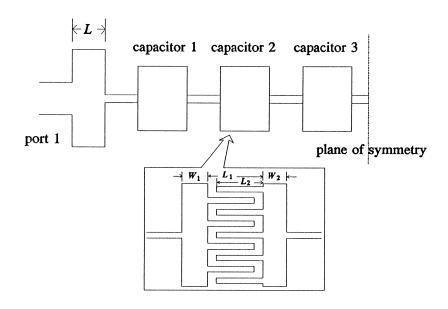
utilizes thin microstrip lines and interdigital capacitors to realize inductances and capacitances of a synthesized lumped ladder circuit
