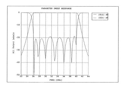
a typical minimax equal-ripple response of the filter was achieved after a series of consecutive optimizations with different subsets of optimization variables and frequency points
