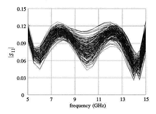
modulus of the reflection coefficient vs. frequency optimization using single-level (component) Q-models 100 statistical outcomes used for yield optimization yield is increased to 86%
