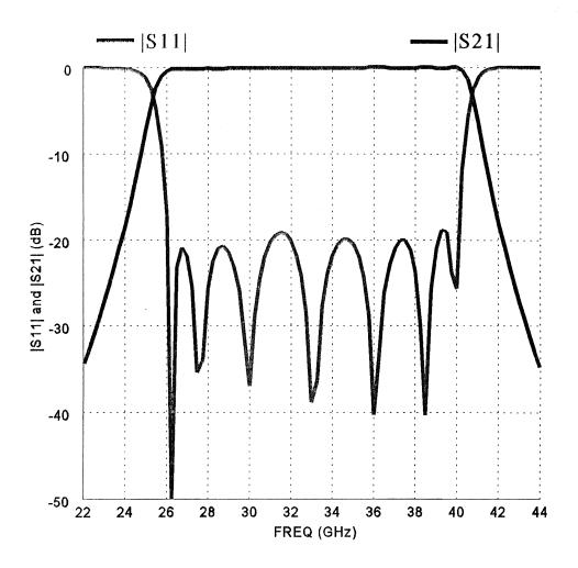
a typical minimax equal-ripple response of the filter was achieved after a series of consecutive optimizations with different subsets of optimization variables and frequency points
