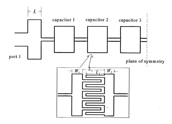
the initial design was obtained by matching a synthesized lumped ladder prototype at the center frequency using  $em^{TM}$
