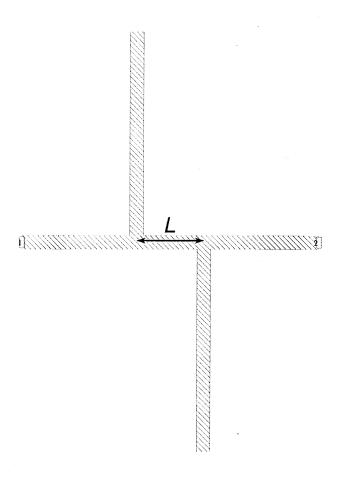
interpolate the parameter L between 30 mils and 35 mils (the grid size is 5 mils).
