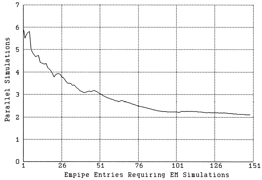
Fig. 6. Utilization of the parallel computing: the cumulative average number of EM analyses run in parallel during the statistical design.
