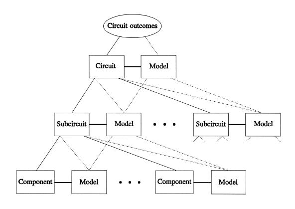
a *Q*-model can be established at any level for some or all subcircuits and components
