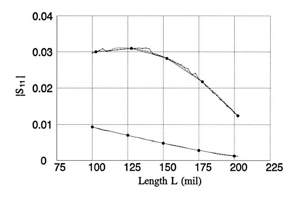
upper curves: the reference data and the responses of the Land Q-models built using the fine simulation and coarse
