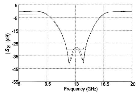
EMF  $|S_{21}|$  response at the EMC minimax solution (dashed line) and SM refined solution (solid line)
