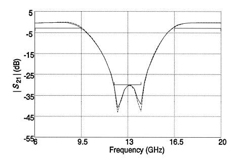
solid line  $|S_{21}|$  at the minimax coarse model solution as simulated using the coarse model
