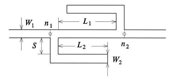
substrate thickness is 5 mil and the relative dielectric constant is assumed to be 9.9
