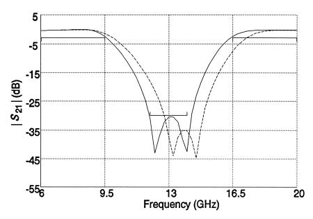
EMC  $|S_{21}|$  response before (dashed line) and after (solid line) EMC minimax optimization
