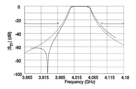
$|S_{21}|$  response of the filter at the optimal OS (dashed line) and EM (solid line) solutions
