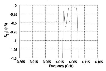
the response exhibits the desired shape with slightly shifted center frequency
