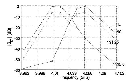
two on-the-grid simulations with  $L_1 = L_2 = L_3 = L = 190$  and 192.5 mil are used to interpolate responses at an off-the-grid (L = 191.25 mil) point; other dimensions are on-the-grid and fixed
