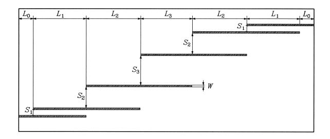
the thickness of the lanthanum aluminate substrate is 20 mil and the dielectric constant is 23.425
