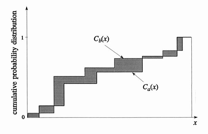
$C_a(x)$  and  $C_b(x)$  are two cumulative probability distributions CPD matching error is indicated by the shaded area
