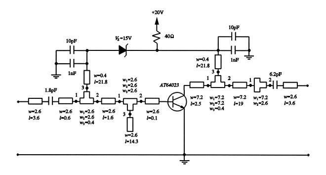
units: mm substrate thickness 1.5 mm relative dielectric constant 4.75 metallization: 35 µm thick copper
