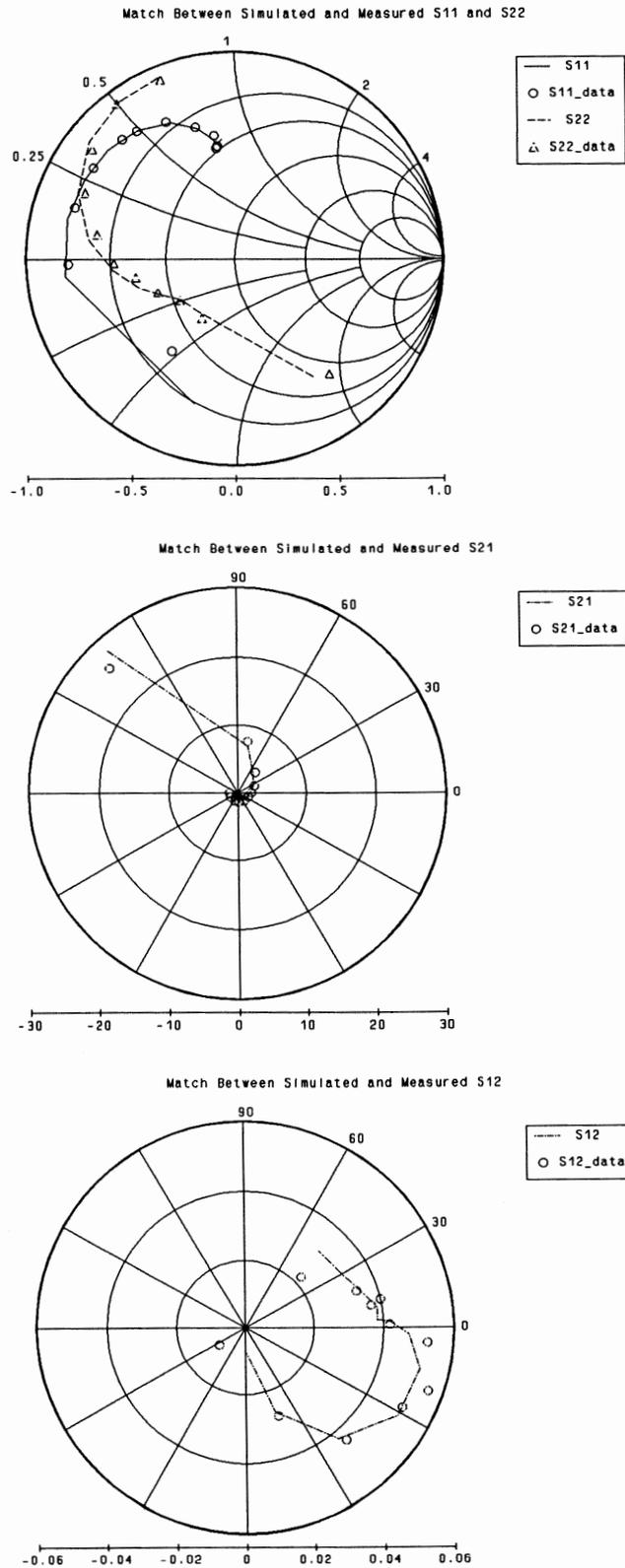
Fig. 2  $S$ -parameter match using the optimized model. The solid and dashed lines are the simulated  $S$  parameters. The  $\circ$  and  $\Delta$  are the measured  $S$  parameters.
