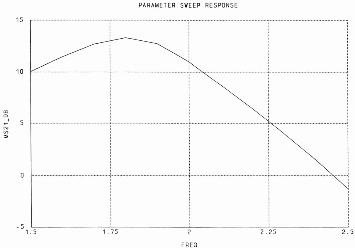
Fig. 3 Small-signal gain of the amplifier with the optimized model.
