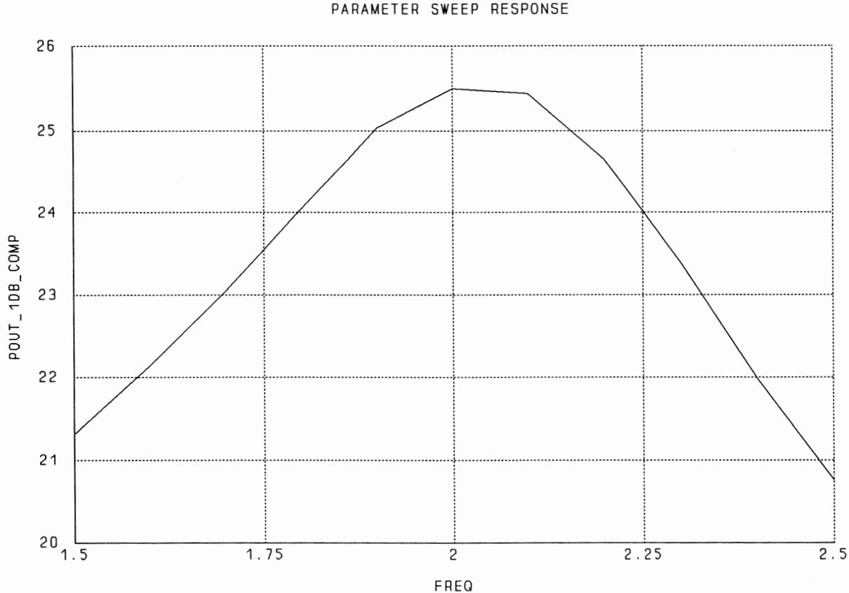
Fig. 4 Output power at 1dB gain compression using the optimized model.
