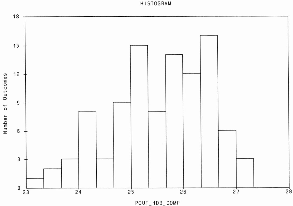
**Fig. 6 Histogram of output power (dBm) at 1dB gain compression at 2GHz for assumed model uncertainty.**
