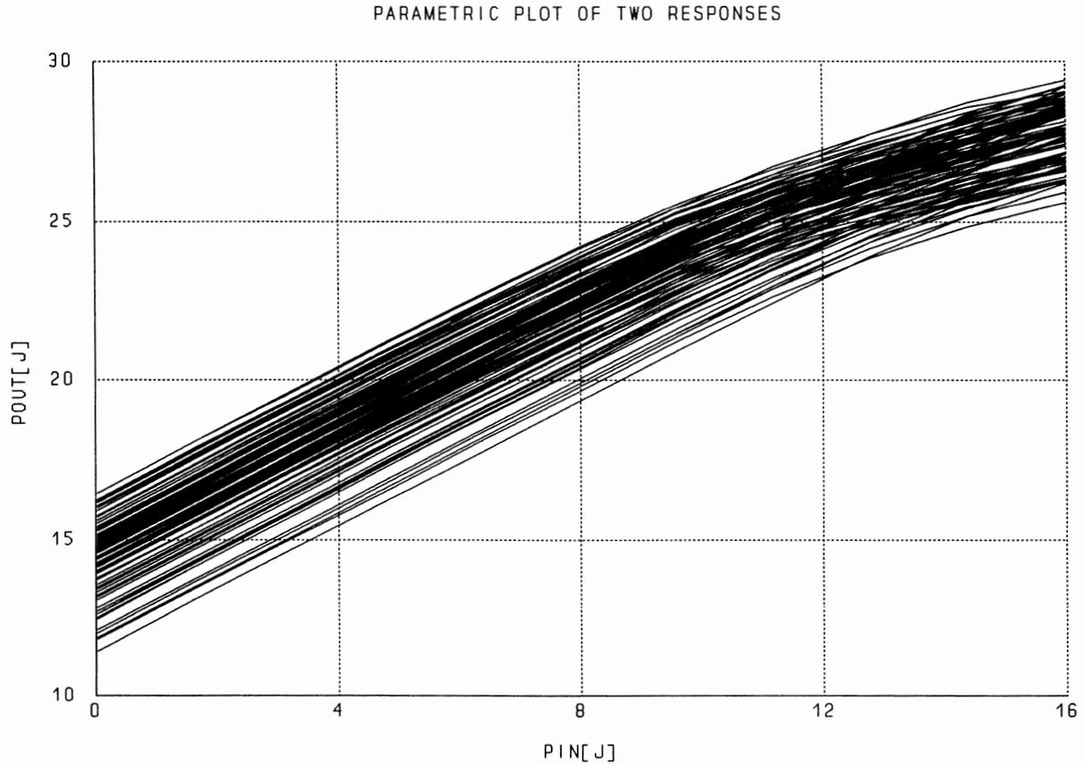
**Fig. 5 Monte Carlo sweep of output power (dBm) versus input power (dBm) at 2GHz.**
