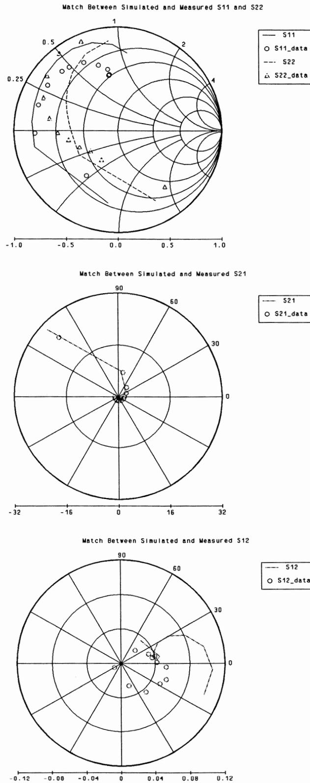
**Fig. 1** *S*-parameter match using the model provided by Avantek. The solid and dashed lines are the simulated *S* parameters. The  $\circ$  and  $\Delta$  are the measured *S* parameters.
