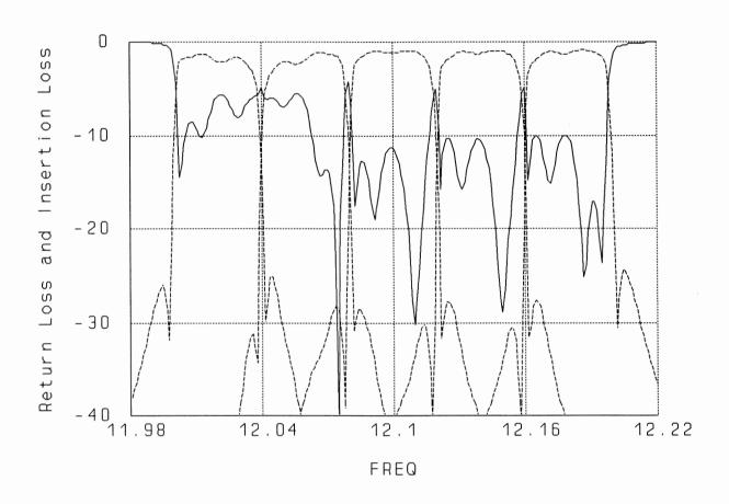
multiplexer responses after minimax optimization with 10 variables: spacings and channel input transformer ratios
