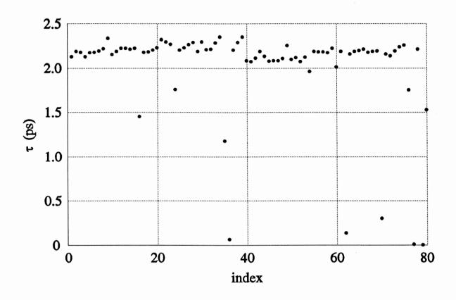
run chart of the extracted FET time-delay τ
