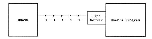
typical READ and WRITE statements are used to receive and send data
