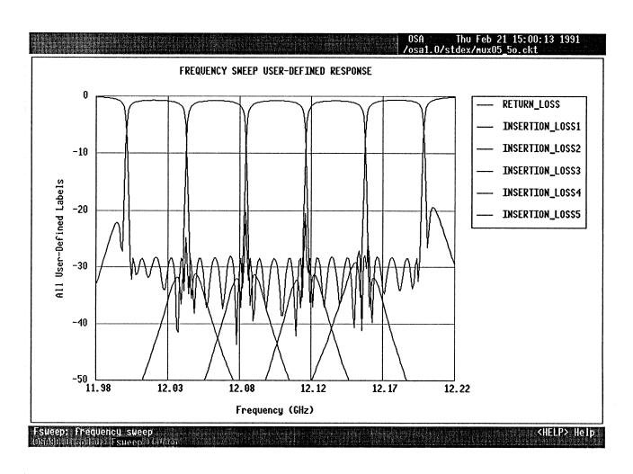
OSA90 and a multiplexer simulator interacted for 3724 iterations
