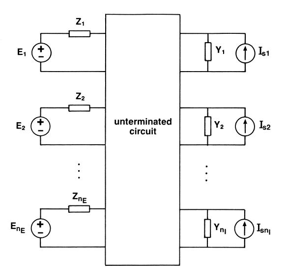
Fig. 3 A representation of a terminated subnetwork. Both current and voltage sources can be accommodated. The overall port sequence is such that ports 1, 2, ...,  $n_E$  correspond to voltage sources and ports  $n_E+1$ ,  $n_E+2$ , ...,  $n_E+n_I$  correspond to current sources. The total number of ports is N, i.e.,  $N=n_E+n_I$ .
