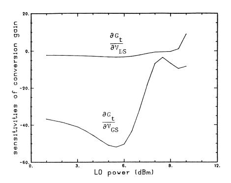
Fig. 6 Sensitivities of conversion gain w.r.t. bias voltages as functions of LO power.
