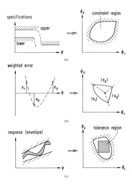
Fig. 1 Some typical design situations. In (a) we have upper and lower specifications on the response function of one independent variable implying a constraint region with respect to the designable parameters. In (b) is shown a weighted error function sampled at three points giving rise to minimax contours. In (c) we have a toleranced design satisfying all performance specifications.
