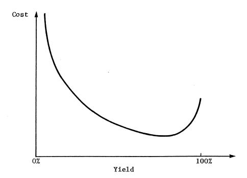
Fig. 2 A possible circuit cost vs. yield curve [2].
