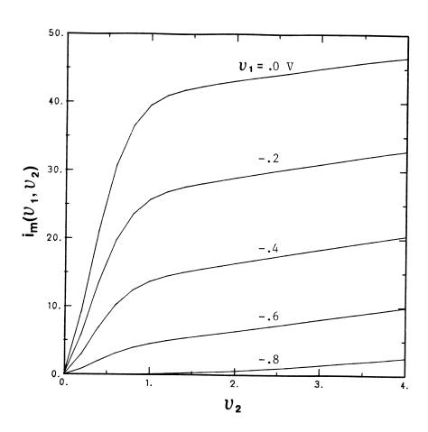
Fig. 5 The DC characteristics of the MESFET model.
