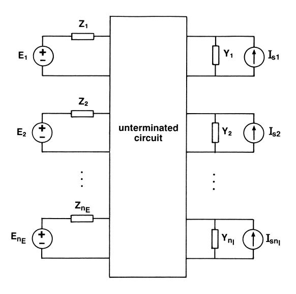
Fig. 3 A representation of a terminated subnetwork. Both current and voltage sources can be accommodated.
