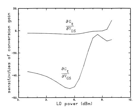
Fig. 6 Sensitivities of conversion gain w.r.t. bias voltages as functions of LO power.
