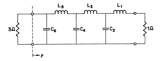
Fig. 1 Six element LC matching circuit used as a test problem for the FTP.
