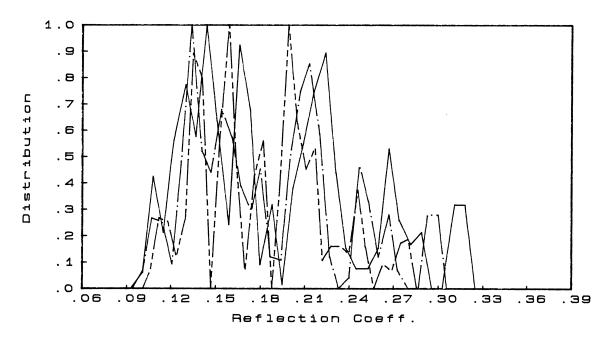
Fig. 14 Vertex analyses comparing the results obtained after nominal design (curve VANOM); after exact FTP design (curve VAOEF21); and after three stages of 5 iterations with problem re-starts when performing a FTP design with the quadratic approximation option (curve VAOESTP). For the latter two designs, Monte Carlo design with 50 random outcomes and 21 sample frequency points were considered.
