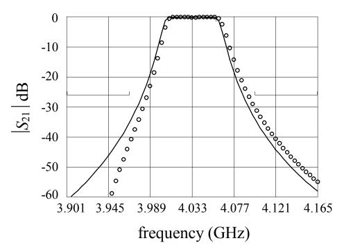
Fig. 17. The optimal coarse model response (—) and the fine model response (o) at the space-mapped design for the HTS filter.
