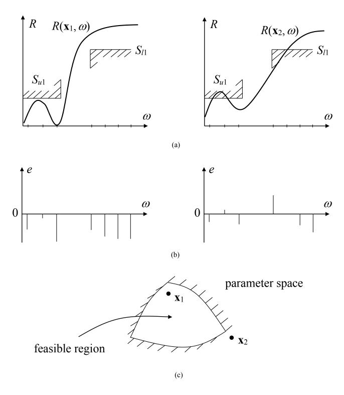
Fig. 1. Illustration of some basic engineering optimization concepts; (a) the responses at a feasible design  $\mathbf{x}_1$  and an infeasible design  $\mathbf{x}_2$ , (b) the error functions at sampled values of the independent parameter  $\omega$  and (c) a possible location of the two designs with respect to the feasible region for a two-dimensional case.
