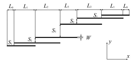
Fig. 15. The structure of the HTS filter [1].
