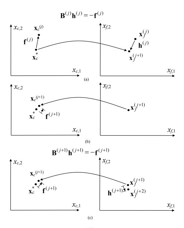
Fig. 5. Illustration of ASM; (a) a new iterate  $\mathbf{x}_f^{(j+1)}$  is obtained, (b) by applying parameter extraction we find that the stopping criterion is not satisfied  $(\|\mathbf{f}^{(j+1)}\| > \varepsilon)$  and (c) the updated matrix  $\mathbf{B}^{(j+1)}$  is used to predict a new iterate  $\mathbf{x}_f^{(j+2)}$ .
