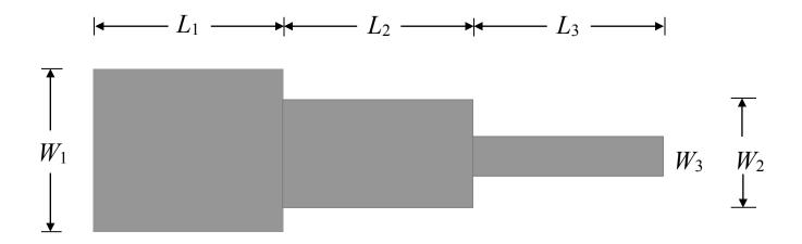
Fig. 6. The three-section 3:1 microstrip impedance transformer [63].
