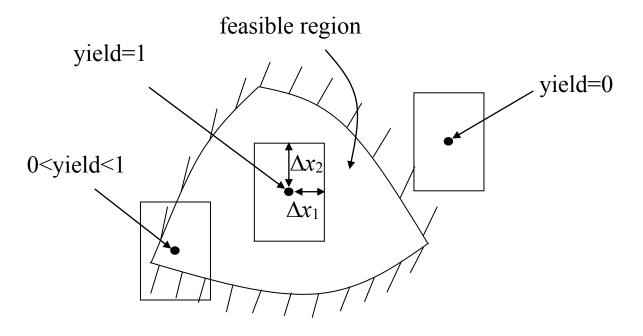
Fig. 2. Illustration of design centering and yield for a two-dimensional problem with manufacturing tolerances of  $\Delta x_1$  and  $\Delta x_2$ . Three different designs are shown; a centered design where all possible outcomes are feasible (yield=1), an infeasible design where possible outcomes are infeasible (yield=0) and non centered feasible design where possible outcomes may be feasible or infeasible (0<yield<1).
