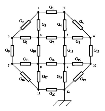
used to demonstrate the  $l_1$  approach to analog fault location
