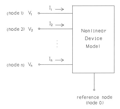
Fig. 1. A generic representation of a nonlinear device model. There are n + 1 nodes in the model. Node 0 is the reference node. The model can be considered an n-port device where port i is between node i and the reference node, i = 1, 2, ..., n.  $V_i$  is the voltage between node i and the reference node.  $I_i$  is the total current flowing out of node i into various branches in the nonlinear model.
