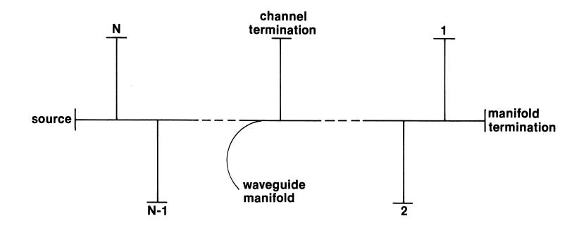
Fig. 1 The basic structure of an N-channel multiplexer
