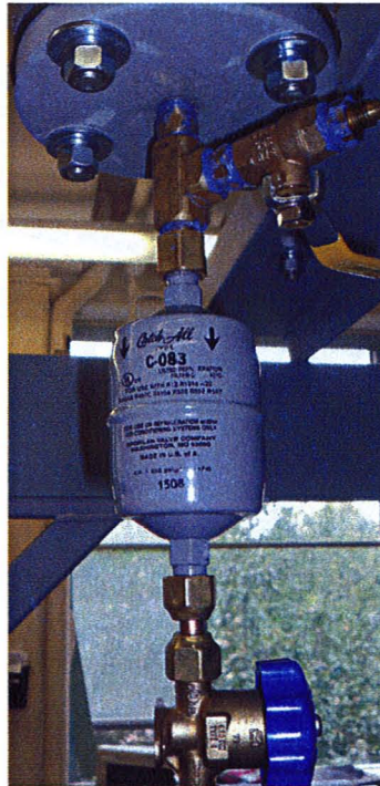
Figure 3-23. Vacuum Tank Purging Port R-134a Filter
