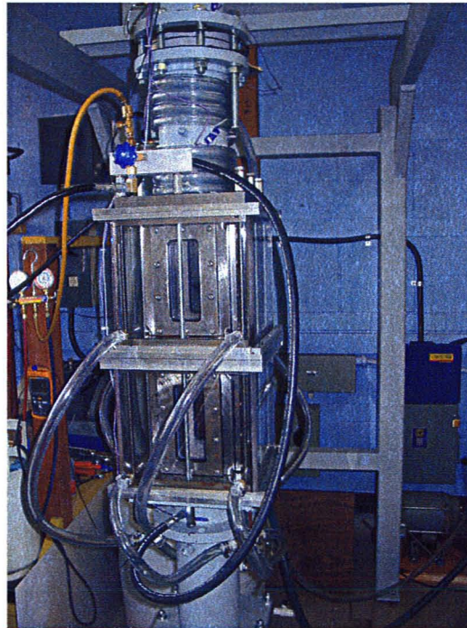
Figure 4-14. Photograph of Cooling System Design
