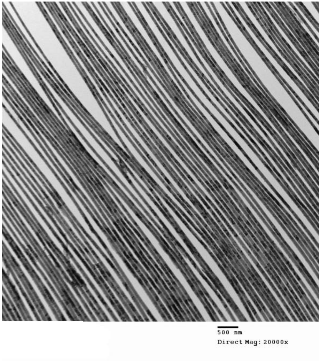
Figure B. 5 TEM of copper nanowires sectioned by controlled chattering at 8 mm/s cutting speed, 40 kHz oscillation frequency and 20nm section feed. Magnification: 20,000 times.
