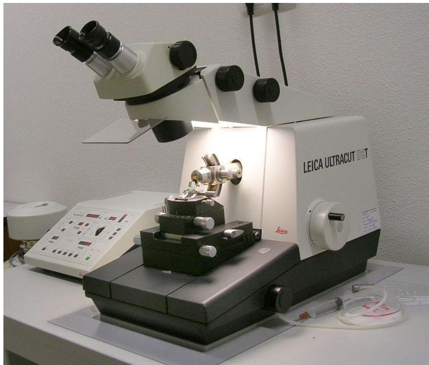
Figure 2.1 Photograph of the Leica UCT ultramicrotome.
