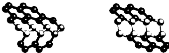
Figure 1.9 Examples of conformations of defect lines that can occur in graphene sheets [YL10,BKK11].
