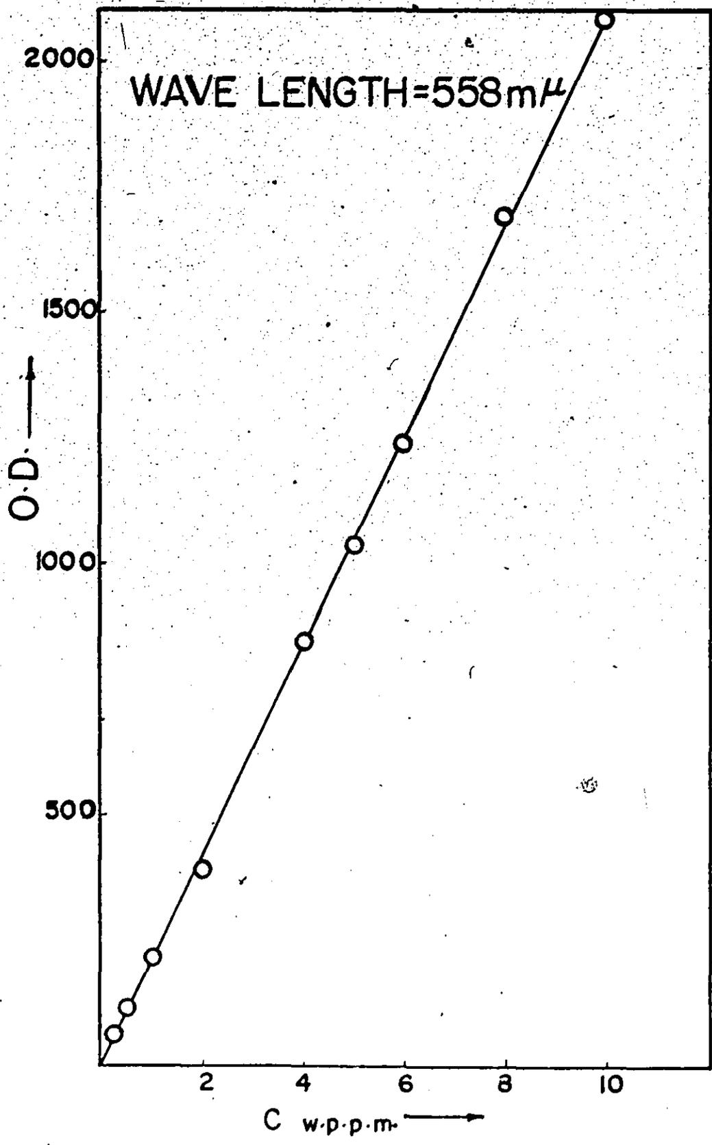
Figure 33. Calibration Curve for the Spectrophotometer.
