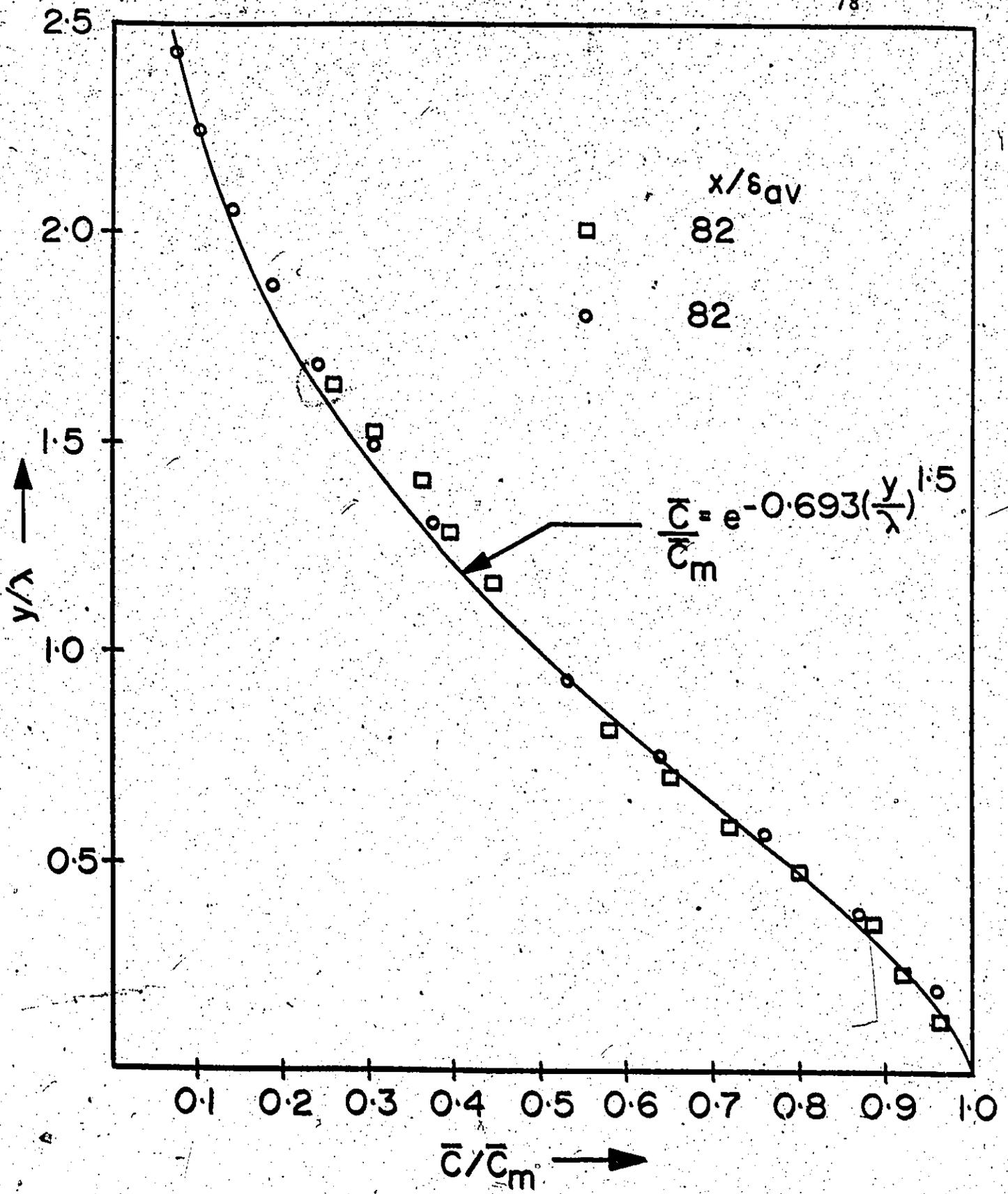
Figure 21. Universal Concentration Profile ( $c_1 = 1500$  w.p.p.m. - Last Location).
