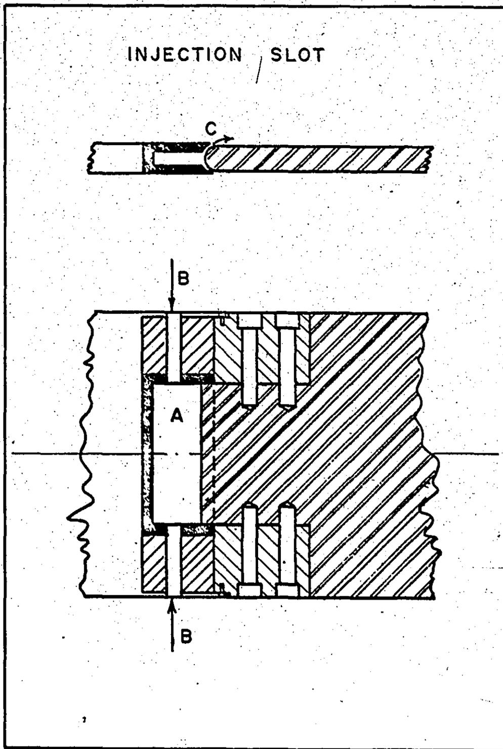
Figure 2. Sectional View of Injection Plechum.
