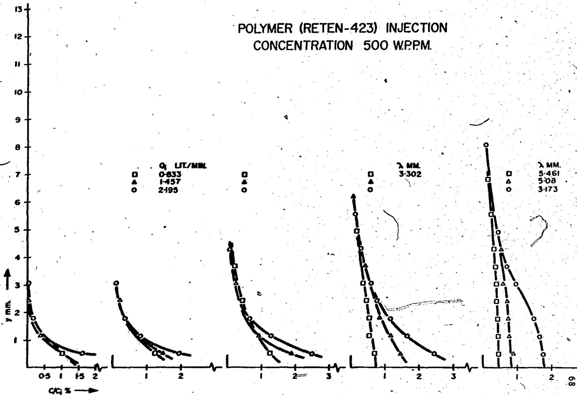
Figure 11. Concentration Profiles ( $c_i = 500$  w.p.p.m.).
