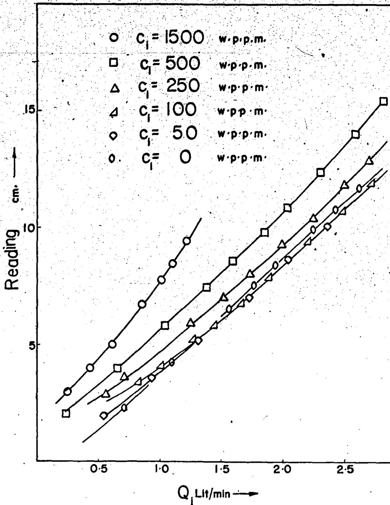
Figure 31. Calibration Curve for the Rotometer.
