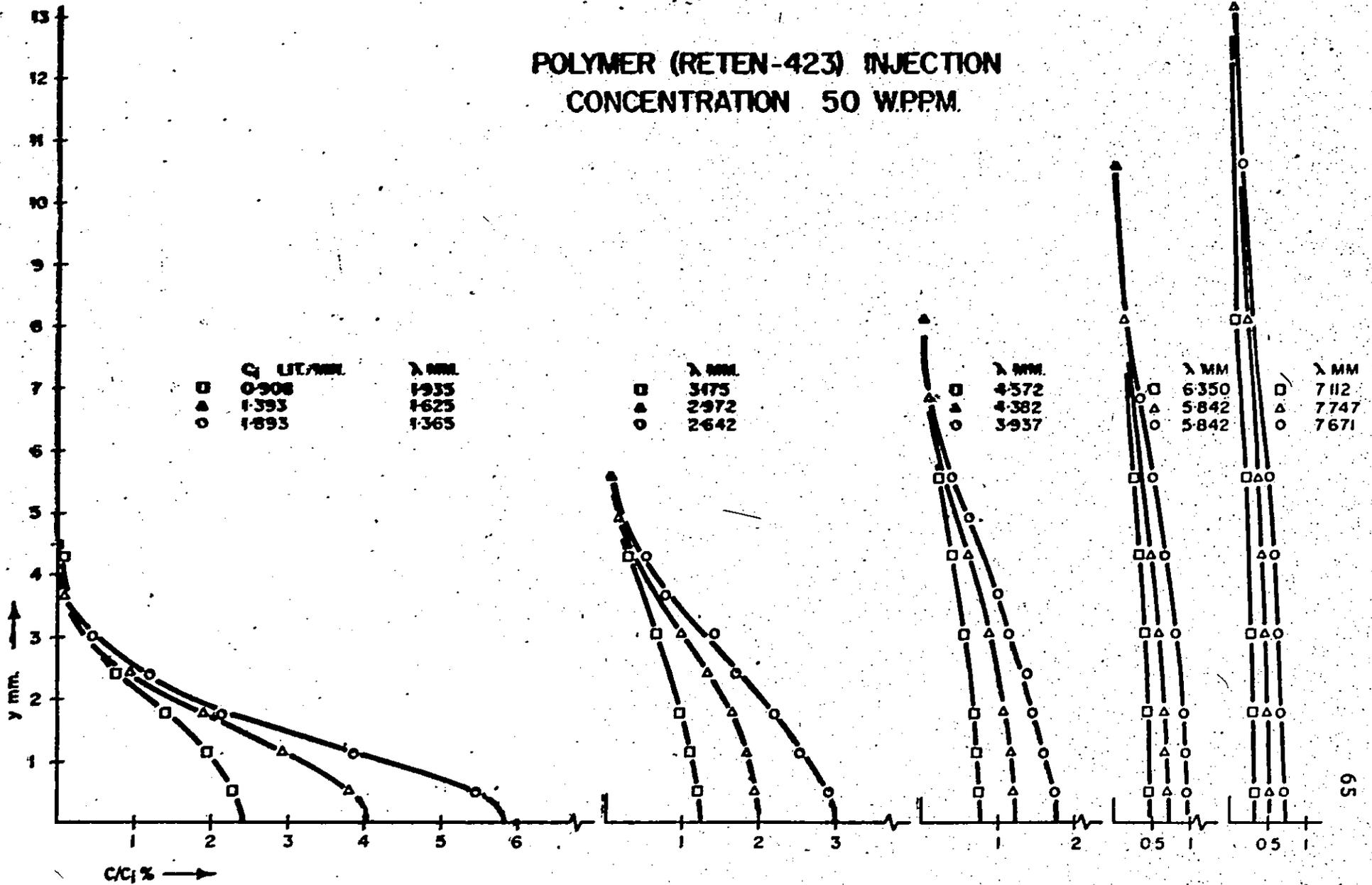
Figure 8. Concentration Profiles ( $c_i = 50$  w.p.p.m.)
