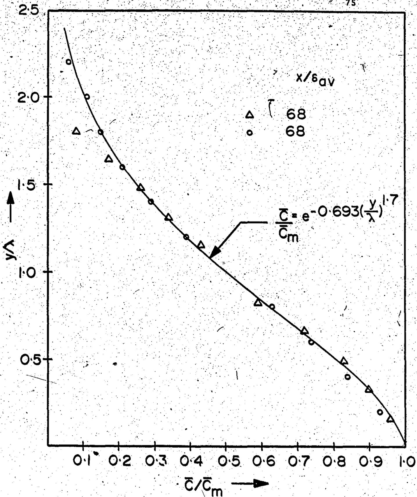
Figuró 18. Universal Concentration Profile ( $c_1 = 250$  w.p.p.m. - Intermediate Zone).
