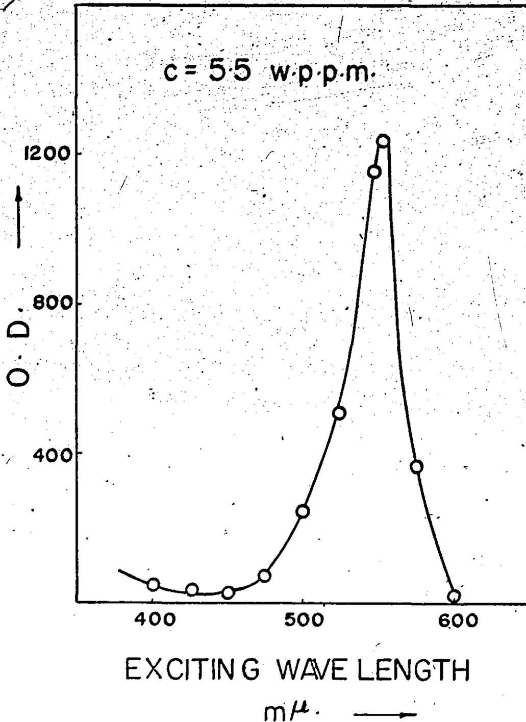
Figure 32. Optical Density (O.D.) vs. Exciting Wave Length.
