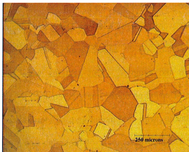
Figure 4.5 Etched Initial Microstructure of 0.4C Alloy
