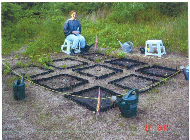
Figure 2.6. a. Design of the remediation grid implemented by Badley (2003) and re-sampled by Mironov (2004). The grid consisted of a 3m x 3m plot of soil subdivided into 1m x 1m squares; 20%-, 10% HP \beta CD solutions were applied 1 pore volume per week for 20 weeks. Control plots received no HP \beta CD applications. Note: figure b (left) is rotated 180°.
