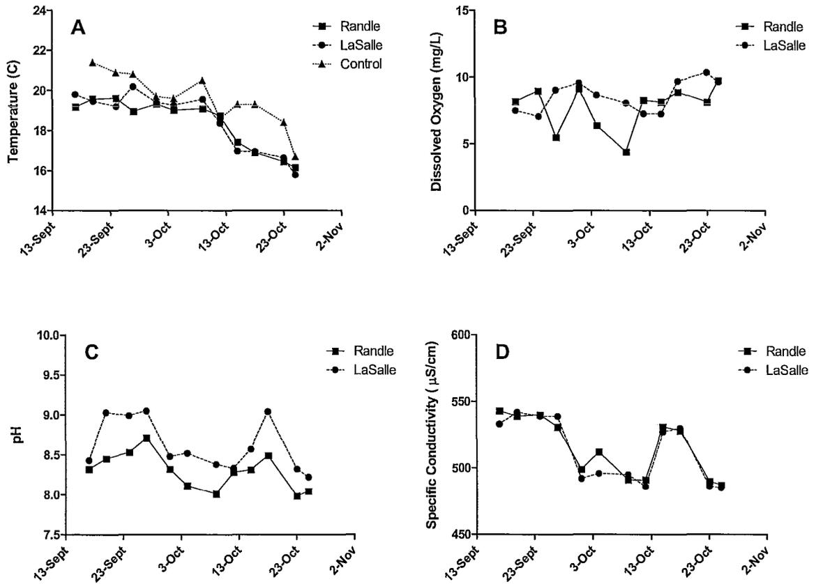
**Figure 2.3:** Temperature (A), dissolved oxygen (B), pH (C), and conductivity (D) profiles during the 6-week field exposure period. All field measurements were taken at cage depth (approximately 7.5 meters deep and 1 meter above sediment).
