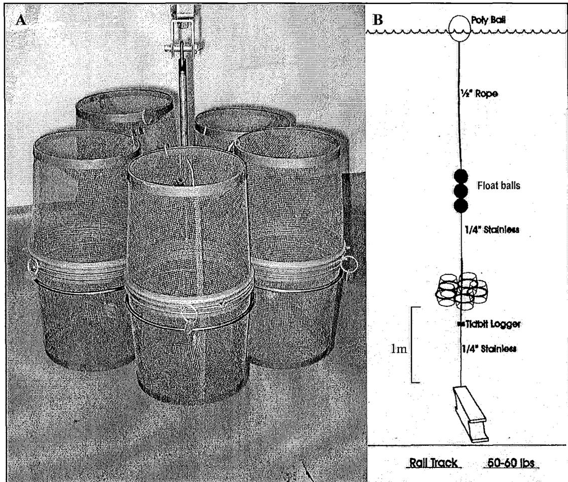
**Figure 2.1:** Each mooring held five modified minnow traps one meter above the sediment surface. A single mooring was used at each field site. **A:** photograph of cages positioned within a mooring. **B:** diagram of the complete mooring as used (not to scale).
