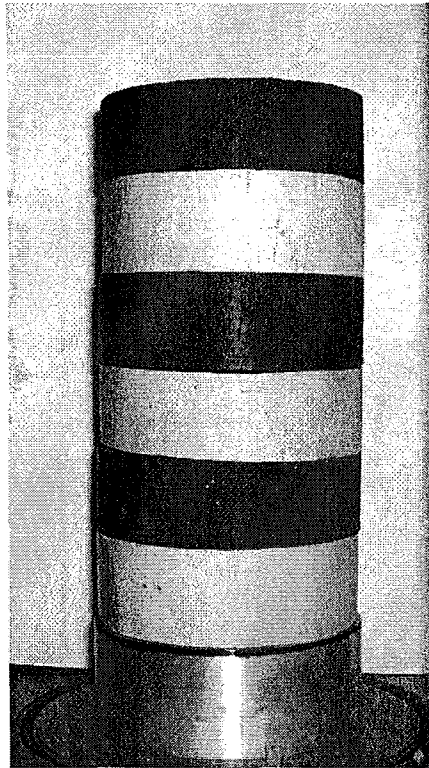
Fig. 3-3 Layered specimens investigated in phase one; consisting 3 layers of Dundas clay and 3 layers of kaolinite; Sample A (7cm in diameter and 10 cm high)
