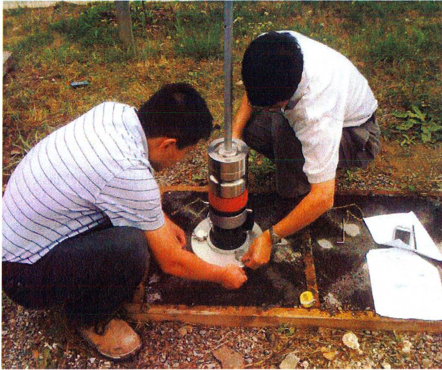
Figure3.1- Dynatest 3031 LWD testing of pavement samples near ADL building, McMaster University (in this photo: Dr. Peijun Guo, McMaster University, and Seth Zhang, John Emery Geotechnical Engineering Limited)
