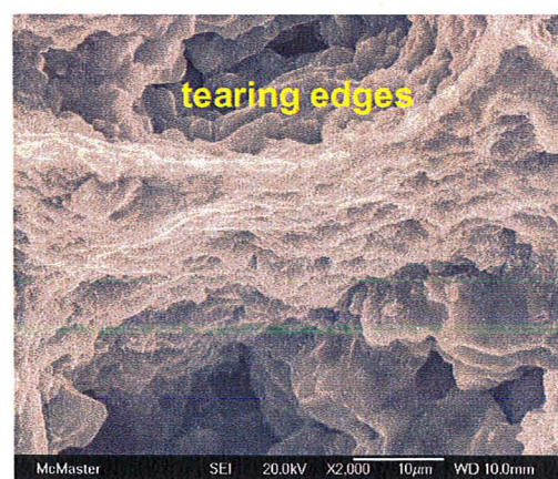
(c) Tearing edges in ‘b’
