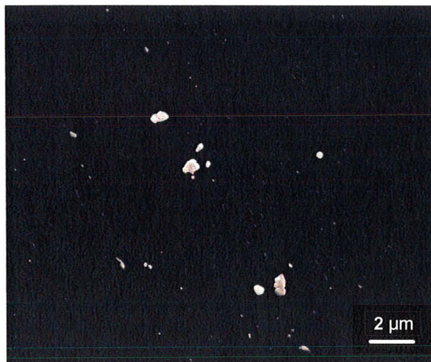
(b) SEM micrograph of AZ31 after annealing at 500°C
