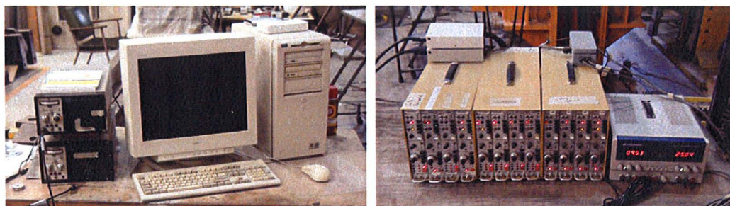
Figure 2.7 Overview of signal control and acquisition equipment: (a) Computer for data acquisition and 406 controllers for vertical and horizontal actuators; (b) Signal filters (12 channels), power supply for LDTs, and sumer box for vertical load cells
