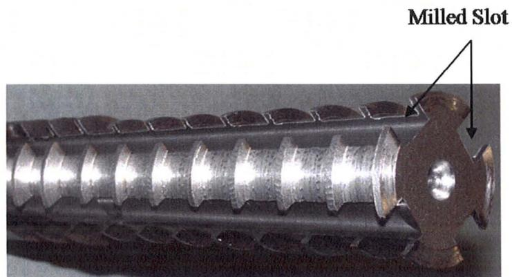
Figure 3.10. Interrupted Cutting Test Sample
