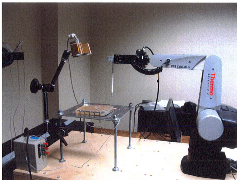
Figure 5.4: Physical experimental setup with robot, camera and planar phantom.
