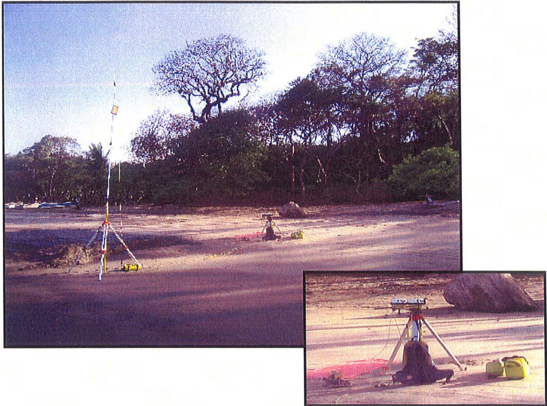
Figure 3.1: Typical deployment of Trimble RTK-GPS system in the center of the beachface at Playa Guiones, Costa Rica. The enlarged image shows the position of GPS receivers for initialization at the base station.
