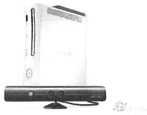
Figure 2.5: Project Natal’s sensor device [Sen09].
