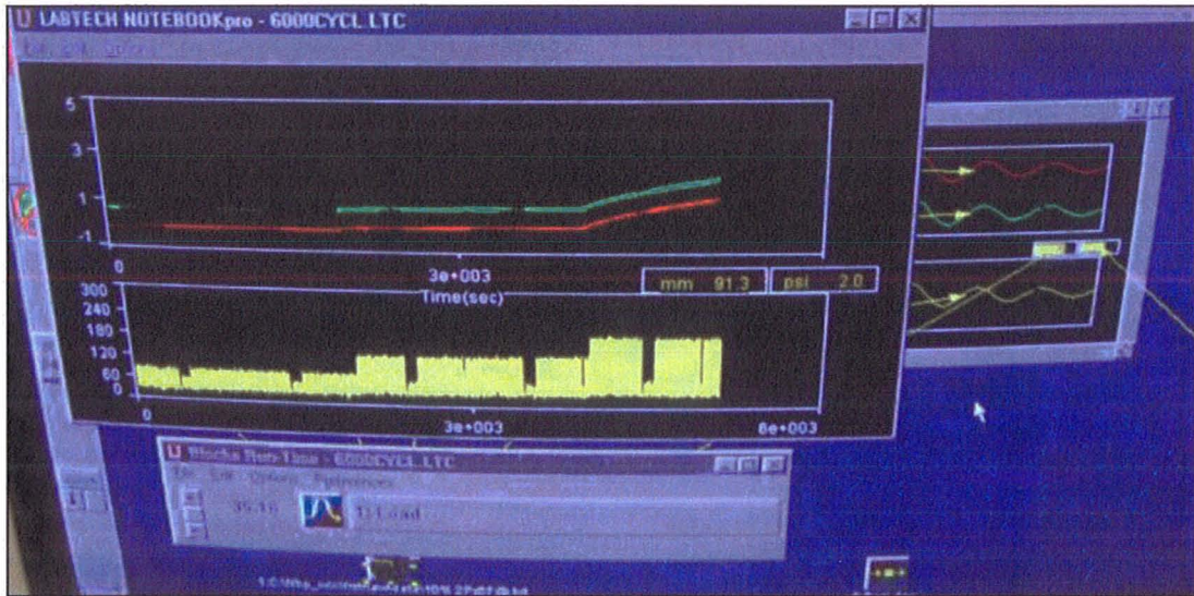
Figure 27 The Accumulative Deformation Observed during the Cyclic Triaxial Test
