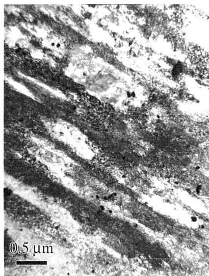
Figure 78: TEM image, Al-4.11at% Mg 4.2K sample, 22,000x magnification
