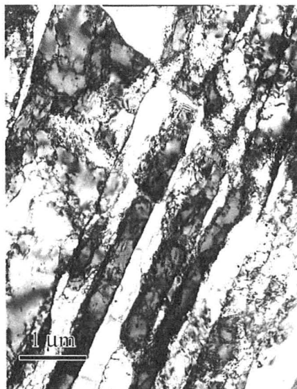
Figure 90: TEM Image, Al-0.36at% Cr 78K sample, 17,000x magnification (B)
