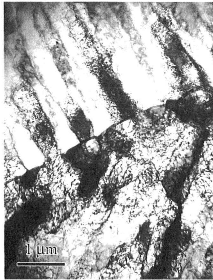
Figure 89: TEM Image, Al-0.36at% Cr 78K sample, 17,000x magnification (A)
