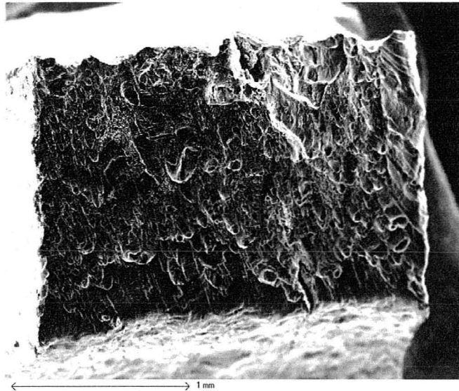
Figure 61: Fracture Surface for 1.08at% Mg sample, 4.2K test, 44.4x magnification
