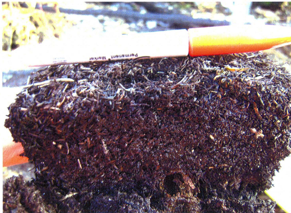
Fig. 4.26 Test #6 (TFABRM), post infiltration excavation – Showing wet (dark) surface wetting and wetting into subsurface brown organic matter
