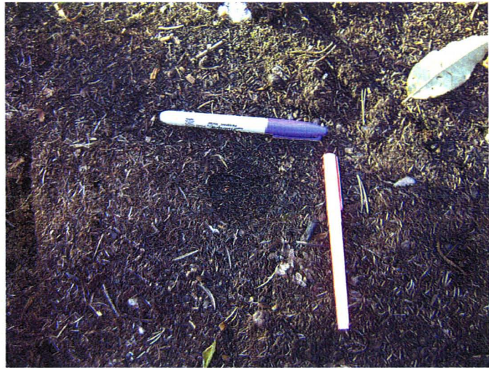
Fig. 4.6 Post infiltration wetted diameter for Brown Materials (BRM), showing no wetting around periphery of disc.
