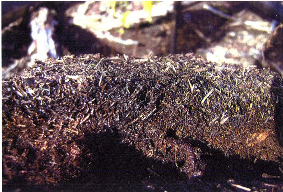
Fig. 4.24 Test #4 (MFN78), post infiltration excavation – Showing wet (dark) surface wetting and wetting into subsurface brown organic matter (approx scale 1cm:1.25cm)
