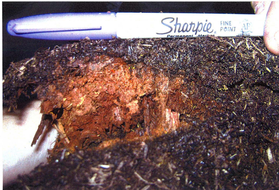
Fig. 4.27 Test #7 (TRBRM), post infiltration excavation – Showing wet (dark) surface wetting and wetting into subsurface wood material
