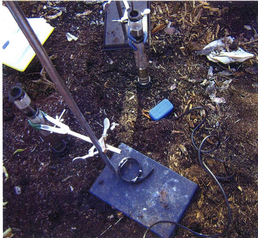
Fig. 4.5 In-progress infiltration tests on Mixed Materials (MM) – left and Char Materials (CM) – right. Blue rectangle = TDR measurement probes.
