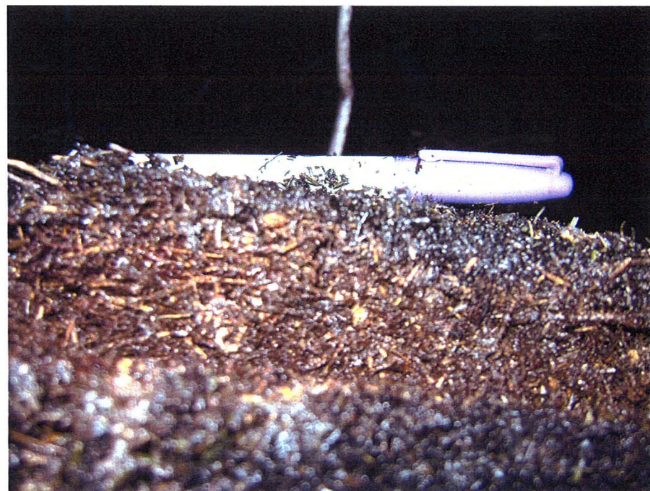
Fig. 4.22 Test #3 (TRCM) post infiltration excavation – Showing char surface material overlying brown organic material, thorough wetting in brown organic layer
