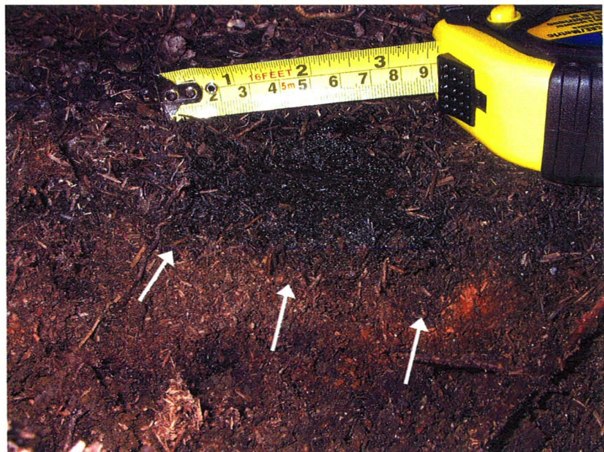
Fig. 4.17 Post infiltration excavation at UPLBRM (Brown Materials) - Showing darkened (wet) area where disc contacted surface, and irregular wetting into subsurface organic materials (arrows) after 69 minutes of testing
