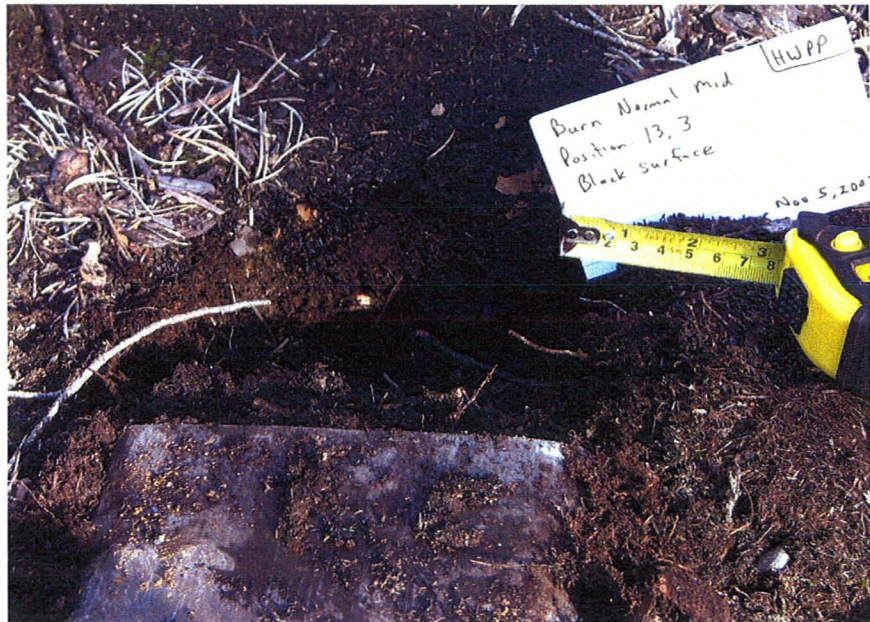
Fig. 4.30 Test #9 (TFAMM), post infiltration excavation – Material surface and brown OM subsurface material
