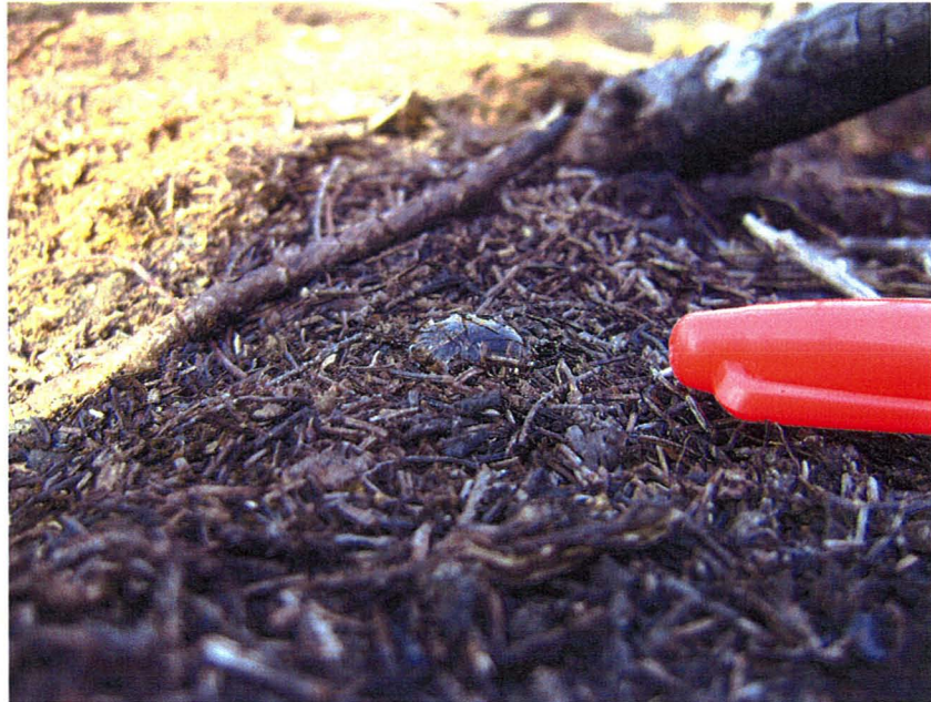
Fig. 4.4 Drop of water on hydrophobic materials; drop size shown is ~5 times the volume of drops used in WDPT tests
