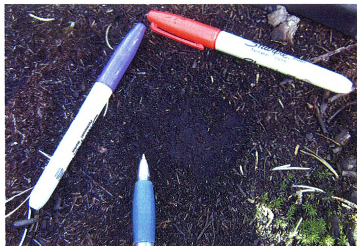
Fig. 4.7 Post infiltration wetted diameter on Char materials (CM). Pen pointing to wet region around periphery of disc area, indicating distribution flow.
