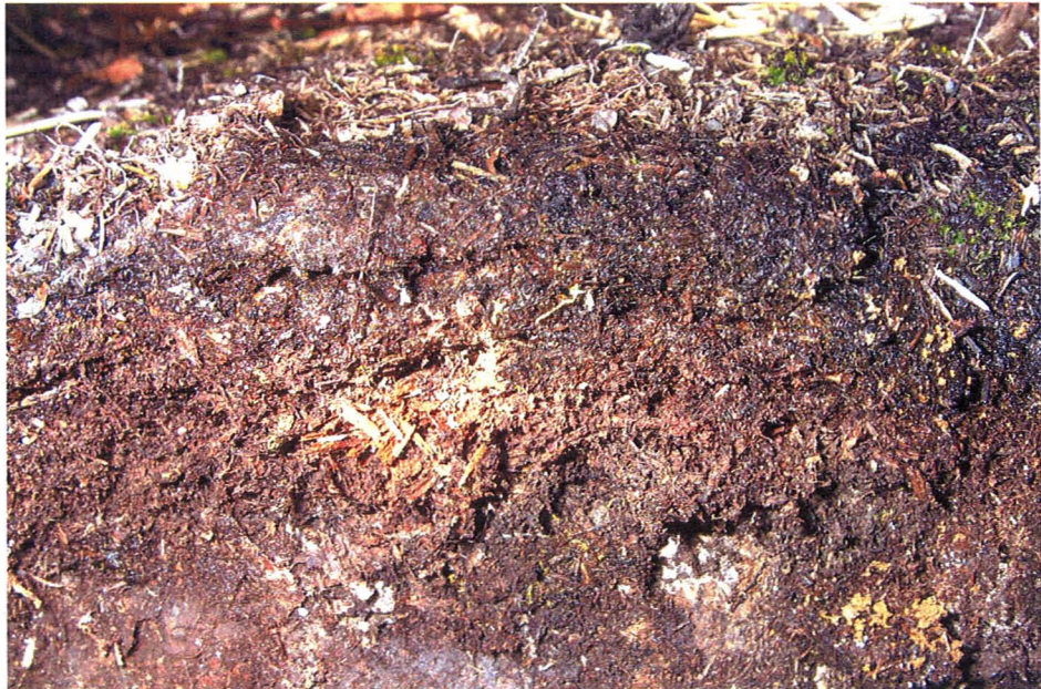
Fig. 4.25 Test #5 (MFN132), post infiltration excavation – Showing wet (dark) surface wetting and wetting into subsurface brown organic matter (approx scale 1cm:1.25cm)
