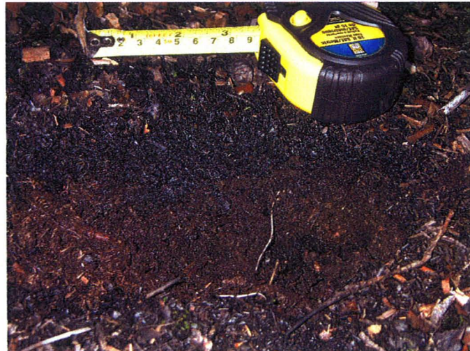
Fig. 4.14 Post infiltration excavation at UPLBTM (Mixed Materials)
