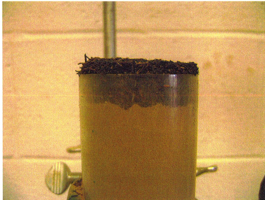
Fig. 3.4 Organic cap material overlying hydrophilic B Horizon Material in column. Column OD = 5cm
