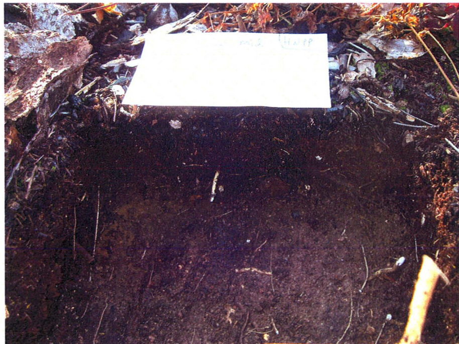
Fig. 4.20 Test #1 (MFN121), post infiltration excavation – Showing char surface material overlying brown organic material
