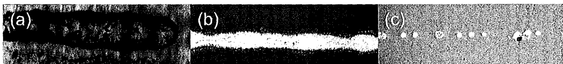
Figure 2.3: Images illustrating silver precursor inkjet printed onto glass microscope slides which have been plasma cleaned (a), plasma cleaned and modified with HMDS (b) and plasma cleaned and modified with OTS (c). Image (a) was taken using a camera built into the Dimatix printer. Images (b) and (c) were taken using an optical microscope.
